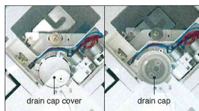
Remove drain cap cover and check the condition. It is necessary to clean-up, firstly remove the rubber stopper to drain water out and secondly remove the drain cap.
